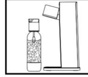
9. Place the bottle and Fizzle-Fuser on a level surface, open the slow release valve, open the slow release valve. Watch the fizz in the bottle. Before the fizz starts to come out the top close the valve and wait for the fizz to settle.
